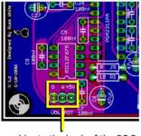
Either solder to the back of the PC Board or to the pins of the potentiometer.
