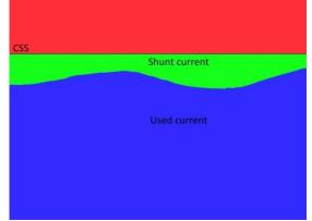
the red zone), it's output voltage will drop at an incredible rate. In most cases this behaviour acts as a decent over-current protection. So if the circuit you are powering develops a short, it's unlikely there will be a lot of damage to the PSU and the rest of your project.
